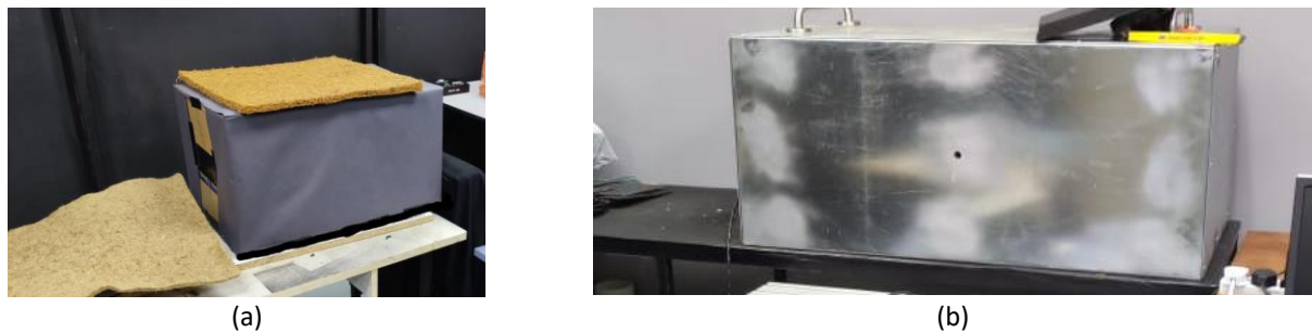
Fig. 3. (a) A wooden soundbox with coconut fibre foam and (b) an aluminium box with insulation foam to suppress the noise from the thermoacoustic test rig
