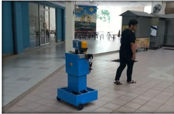
Figure 11. The TR successfully detects and follows the targeted person with the correct measurement.
