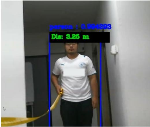
Figure 6. Experiment setup for person detection and distance estimation.
