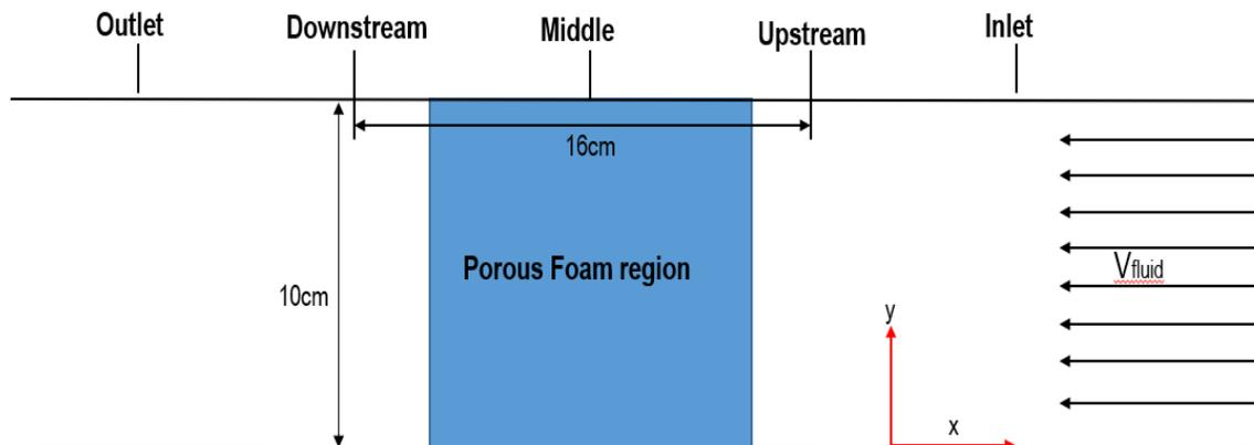
Figure 5: Schematic diagram wind tunnel test section.
