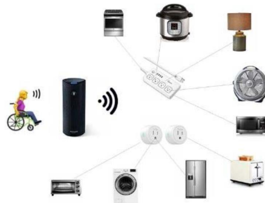
Fig. 4. Example of using IoT to remotely control household devices by elderly and disabled persons [38].
