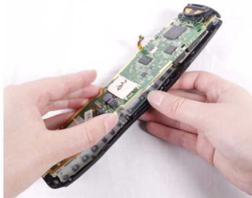
Figure 7. Removing embedded parts in remote control.
