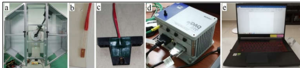
Figure 3 Apparatus and instruments used in Charpy test: (a) 250 J Charpy machine, (b) strain gauge, (c) strain gauge glued onto the impactor, (d) data acquisition system (eDAQ), (e) laptop computer for result display.
