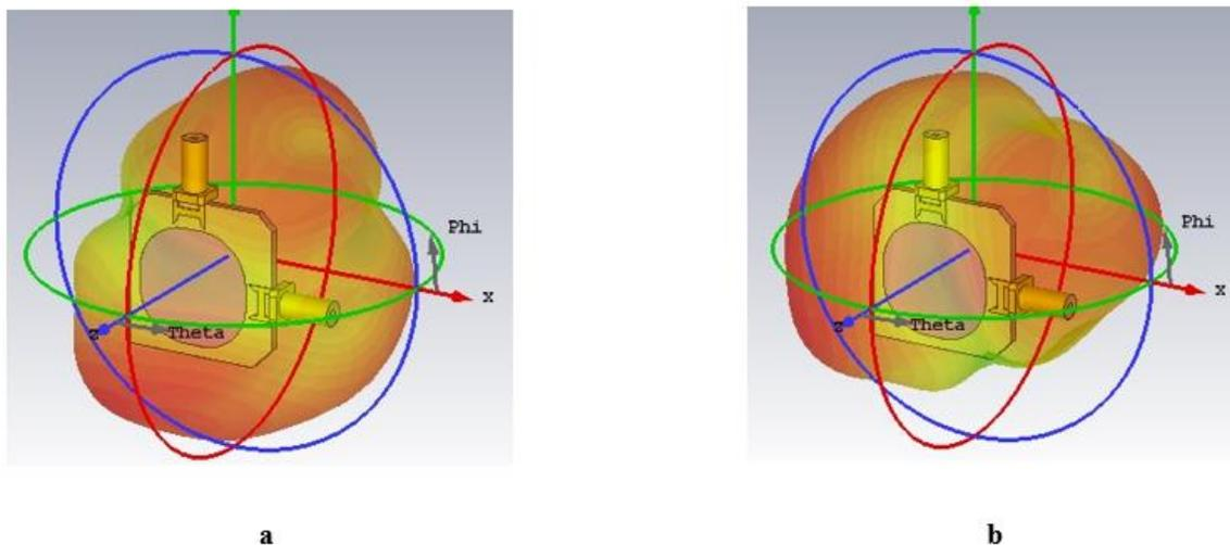
Fig. 6. The dual polarized radiation's 3 dimensional; a) port\_1 and b) port\_2
