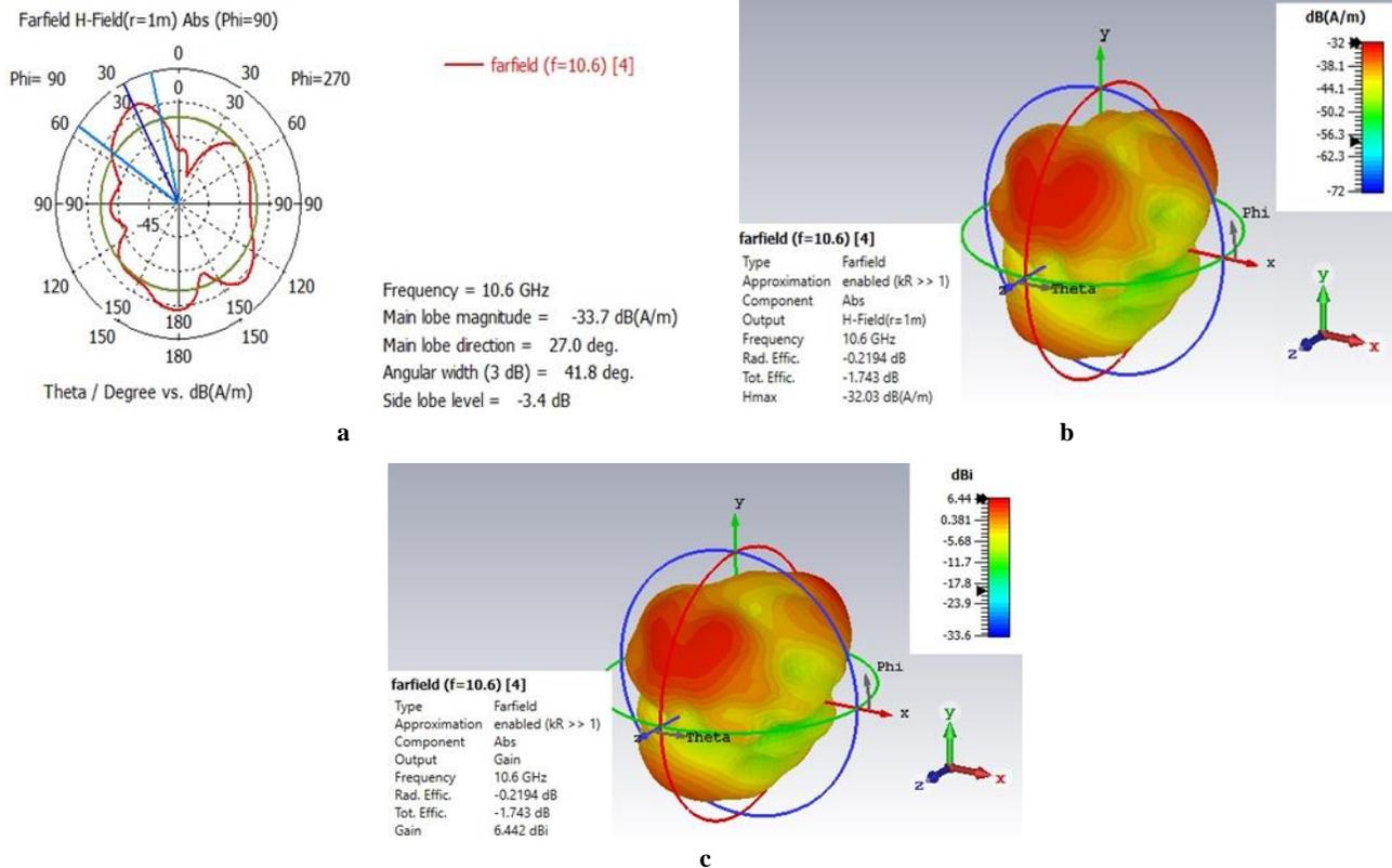
Fig. 11. Radiation Pattern of the MIMO Antenna System a-2D, b- 3D, and c- Gain
