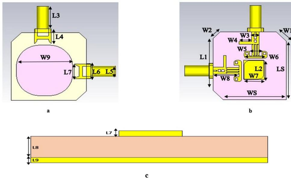
Fig. 1. The antenna design; a) frontal view, b) back view, and c) Side view
