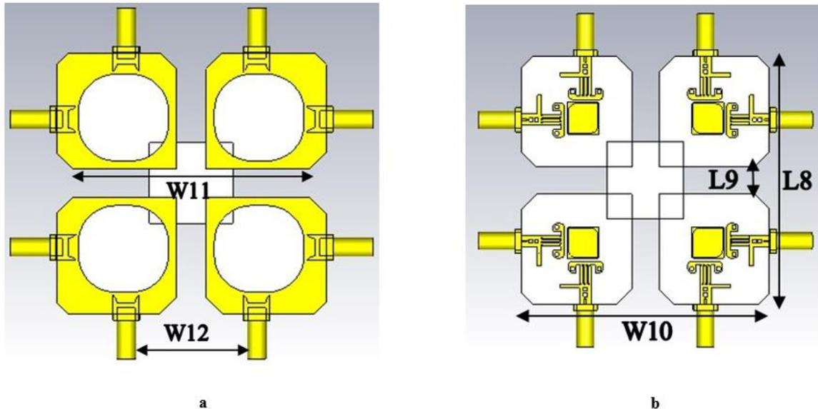
Fig. 2. The MIMO antenna design; a) frontal view, and b) back view
