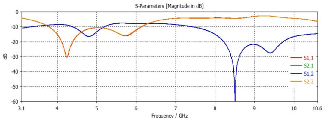
Fig. 3. Details of S-Parameter for a single antenna
