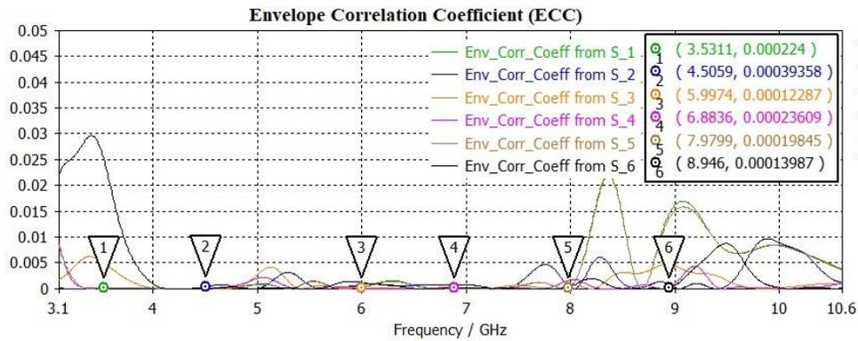
Fig. 9. Details of ECC for MIMO antenna
