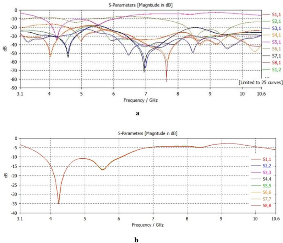
Fig. 7. The S-Parameters for MIMO system a- S Parameters and b- mutual-coupling
