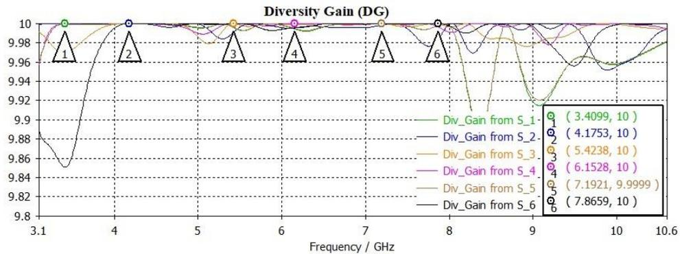
Fig. 10. Details of DG for MIMO antenna
