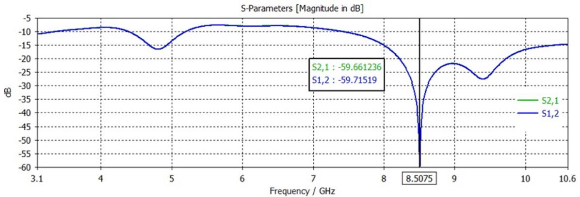
Fig. 4. The mutual coupling coefficient for a single antenna
