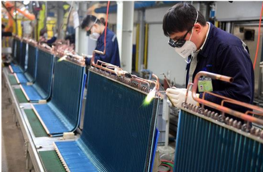
Figure 1.3: Prolong standing position of worker at an air conditioning copper pipe welding assembly line. Taizhou Youyi Automation Technology Co., Ltd. China (2023)
