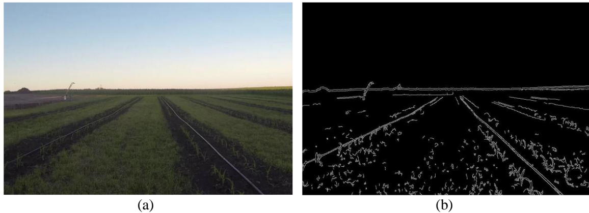
Fig. 15. (a) Image Input of edge-of-row detection and (b) Canny edge detection result [84]
