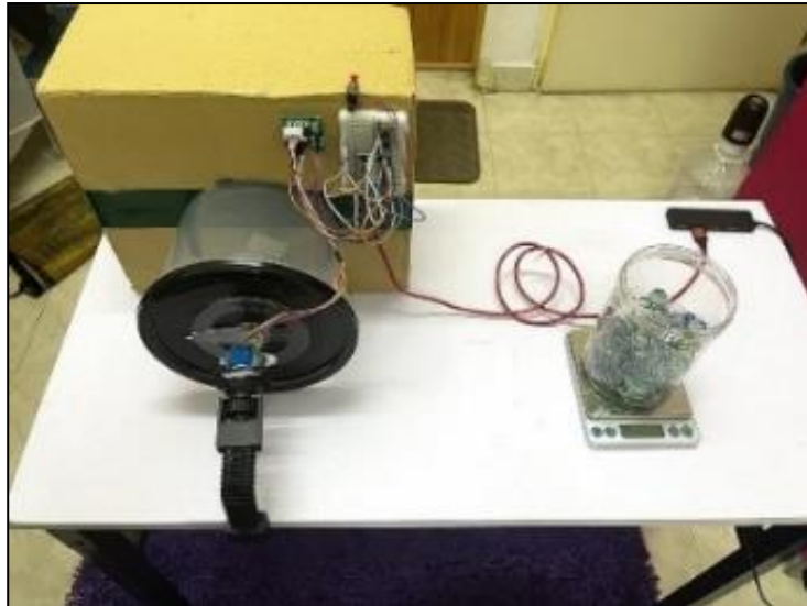
Figure 3: Unipolar 28BYJ-48 Stepper Motor Setup
