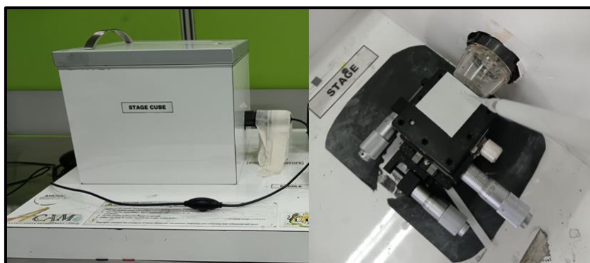
Figure 4 : The self-fabricated contact angle measurement set-up.
