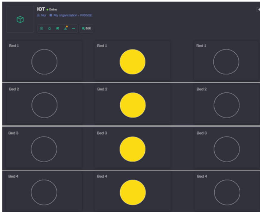
Figure 9: Dashboard indicating beds needing cleaning
