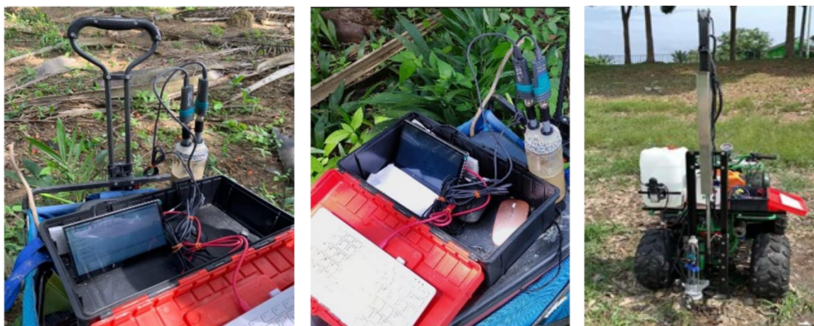
Figure 5. Deployed multi-soil and environment sensor on the field
