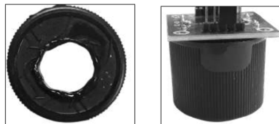
Fig. 4. Setup of tip area for TCS3200
