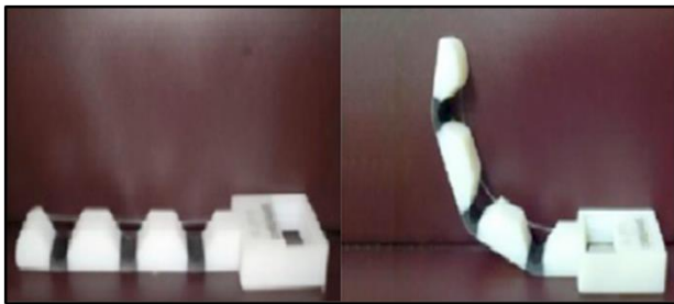
Figure 11 Soft Robotic Finger [2]
