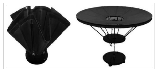
Figure 10 4D Printed Reflectors Used in Spacecraft [54]
