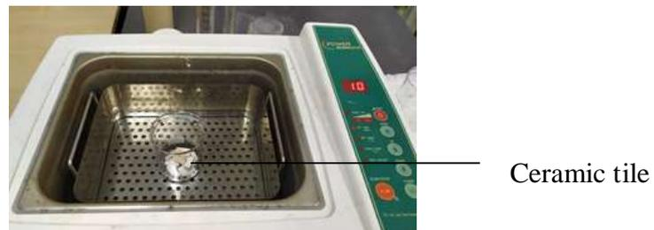
Figure 3.3: Cleaning process of unglazed and glazed ceramic tiles in ultrasonic bath
