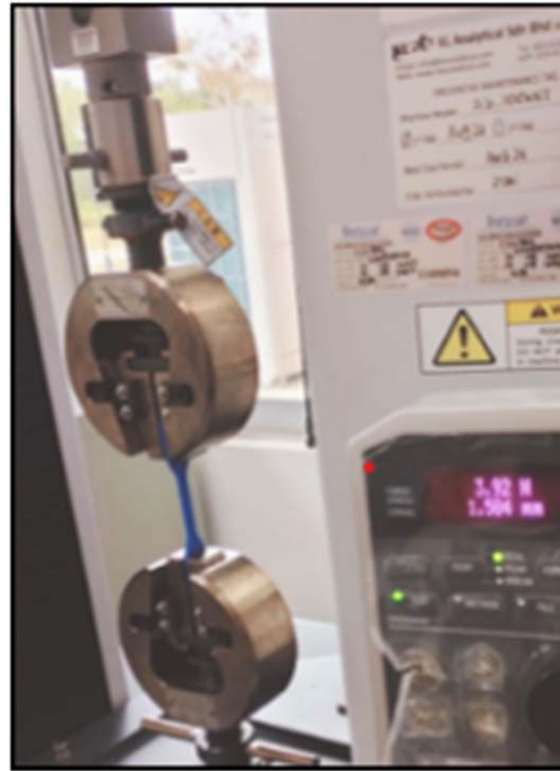
Figure 7. Tensile test sample in universal tensile machine.
