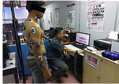
Fig. 4. Interfacing process between EMG sensor and Myon sEMG software [12]
