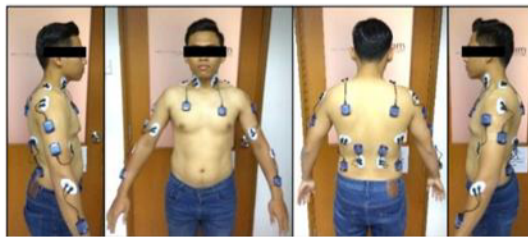
Fig. 3. A Motorcyclist Respondent being fixed with sEMG Electrodes and Transmitter [12]
