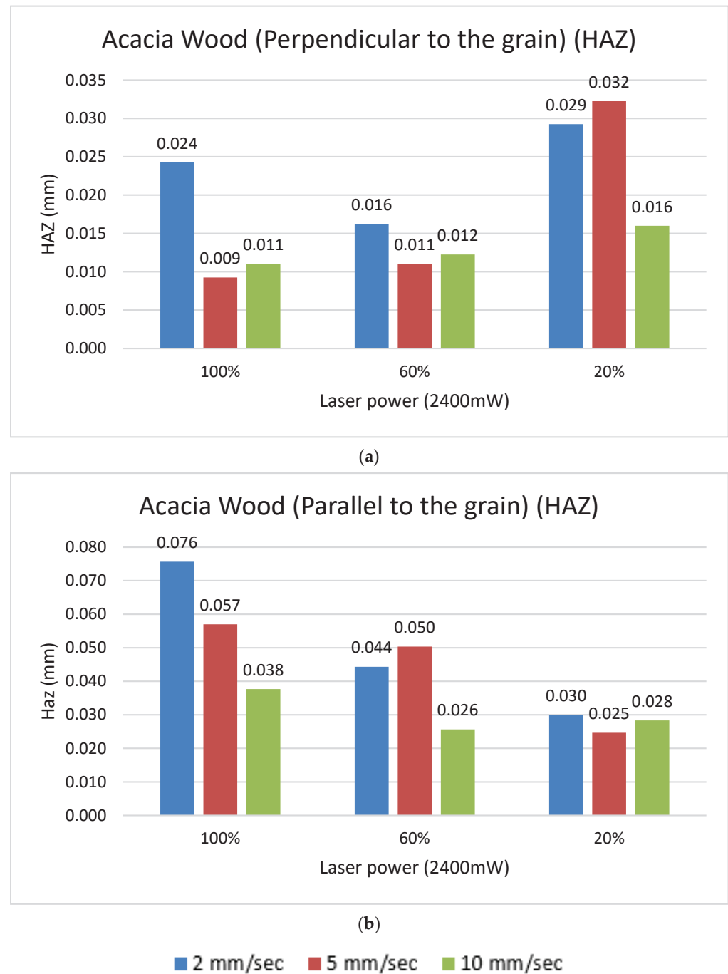
Figure 6. The effect of HAZ at laser power and speed on Acacia wood with direction: (a) perpendicular to the grain and (b) parallel to the grain.
