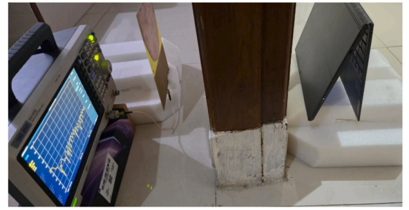
Fig. 13. Experiment set up for Through Wall Radar application.
