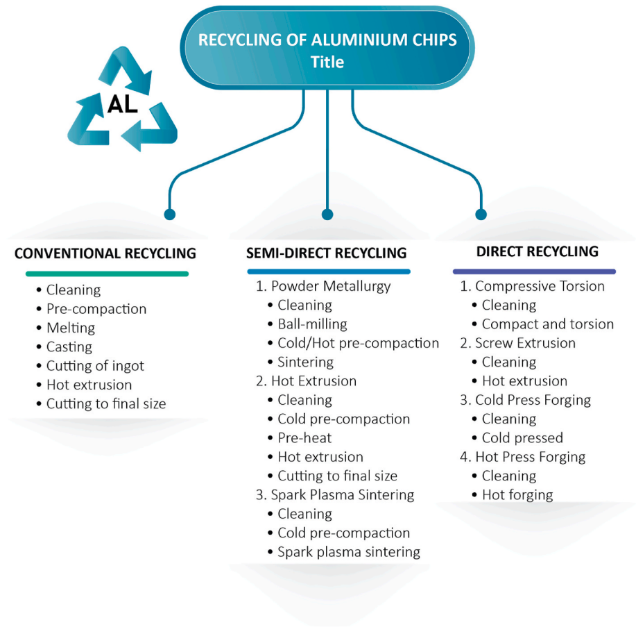
Fig. 4. A comparison of conventional, semi-direct recycling and direct recycling techniques for aluminium alloy chips.
