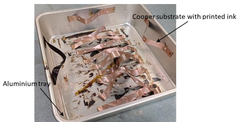
Fig. 18. GNP/Ag conductive ink for curing process
