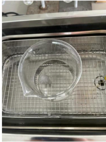
Fig. 3. Melt the PCM into the liquid stage
