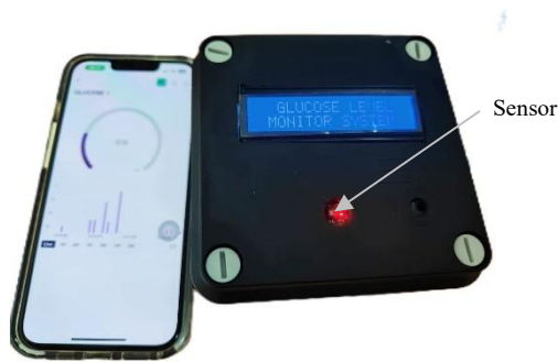
Fig. 7: Prototype for the Non-invasive Glucose Measurement System
