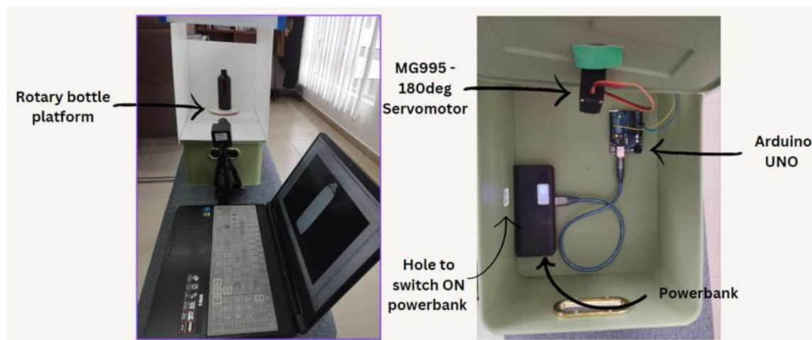
Figure 2 Rotary platform and internals of the electronic case holder.
