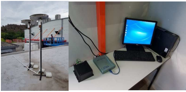
Fig. 3. Capacitive antenna with slow and fast electric field sensor attached, PicoScope 4000 series, AC-DC power supply with -12VDC +12VDC and desktop computer with PicoScope 6 software installed.
