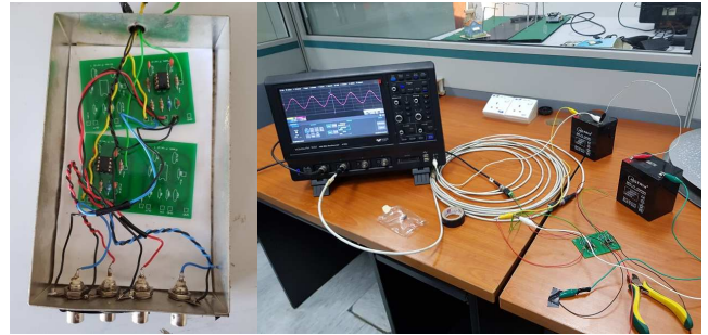
Fig. 2 Slow and fast electric field sensors, calibrated using LeCroy Wavesurfer 3054 oscilloscope.
