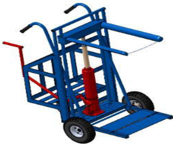
Figure-6. Detailed design of the proposed trolley.
