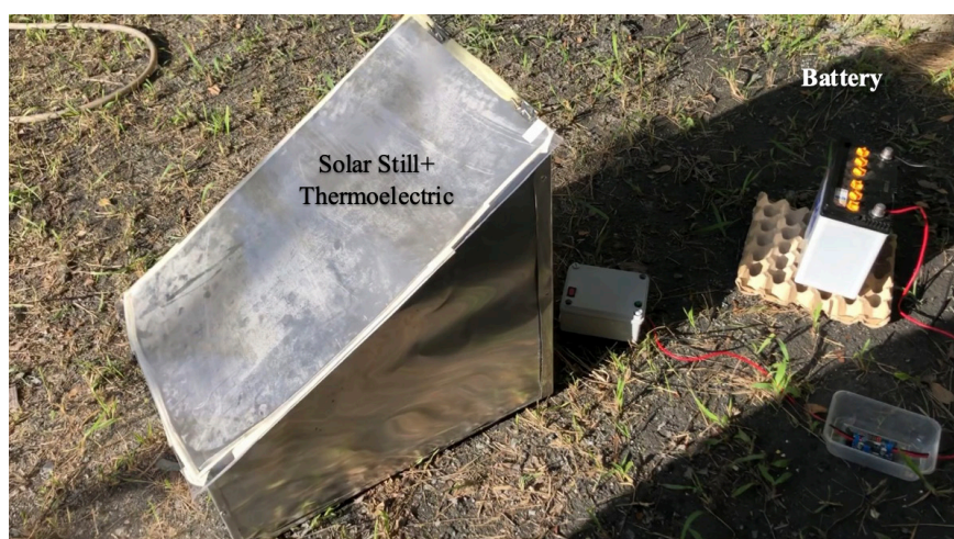
FIGURE 3. Solar Still with Thermoelectric System
