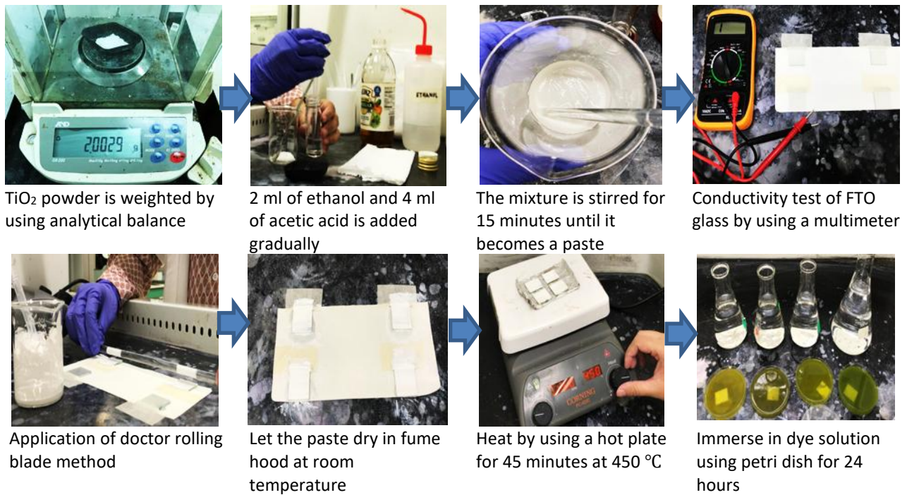
Fig. 3. Preparation of TiO 2 layers and photoelectrode
