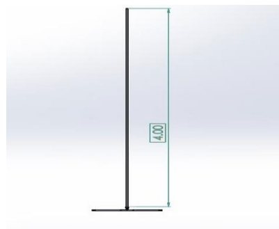
Figure 3. PVC pipe for water head simulation.
