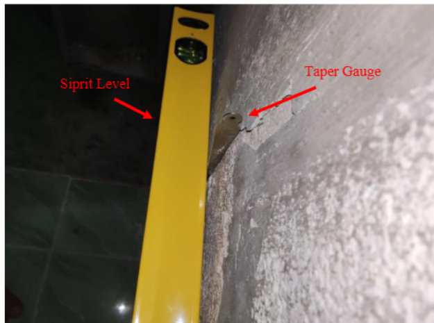
Figure 10 Conventional method of assessing wall evenness
