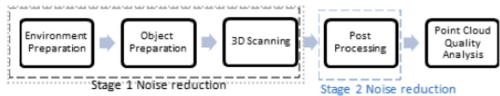
Fig. 9 Flowchart of proposed methodology for noise reduction
