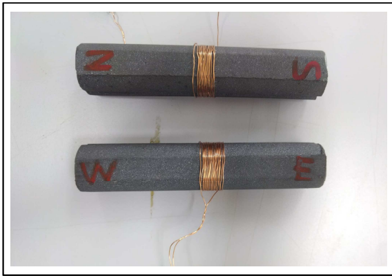
Fig. 1. Ferrite core coils with 20 turns winding.
