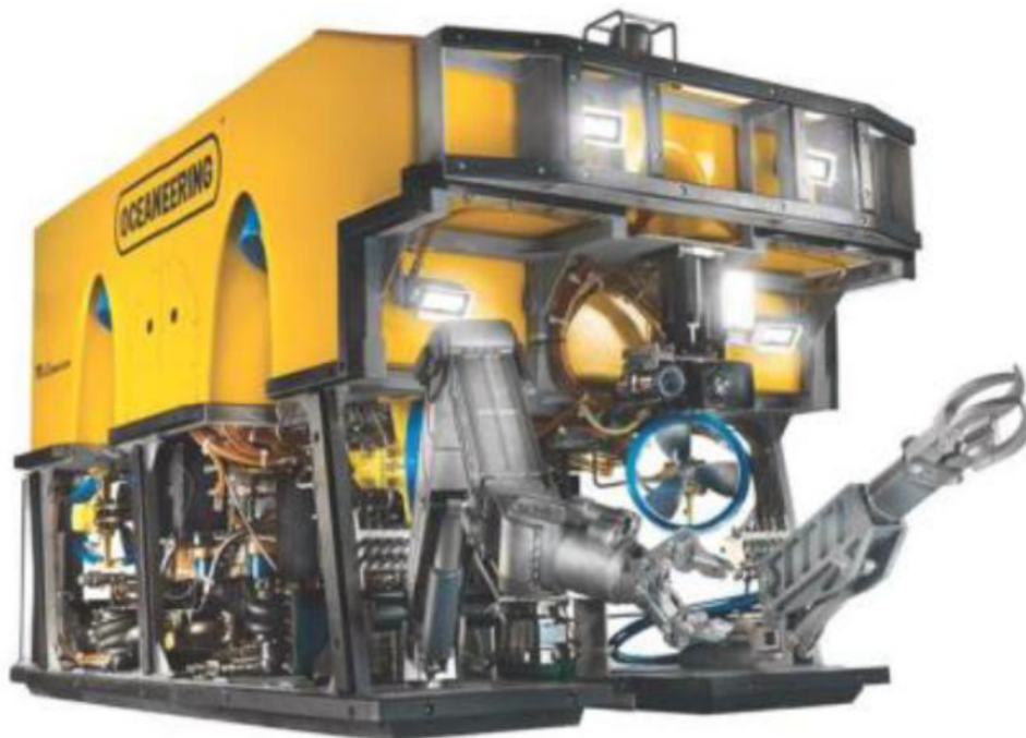
Figure 1. Work class ROV with an open box frame ROV design [12]
