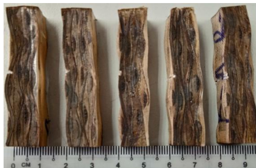
Fig. 1. Woven rattan fibre reinforced polymer before impact
