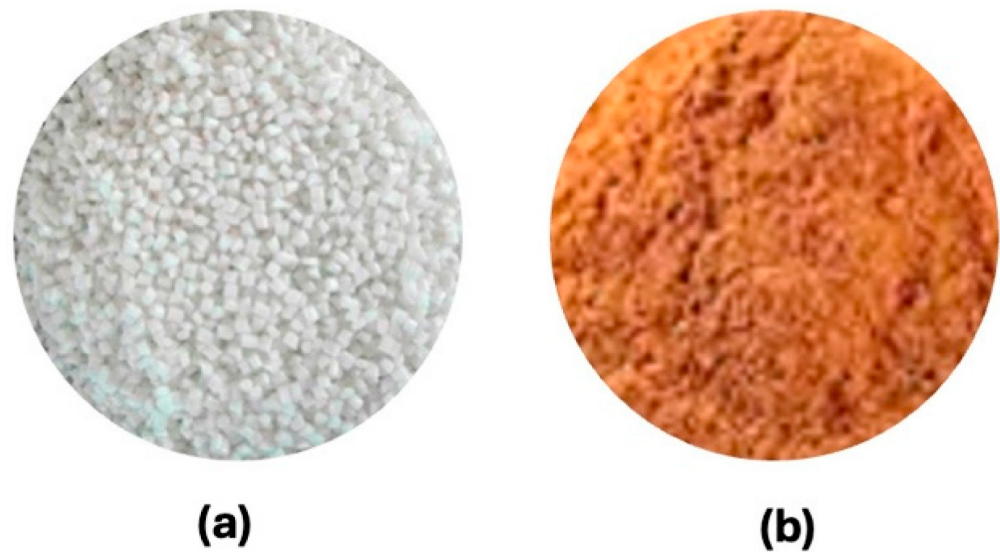
Figure 1. (a) PP pellets (2.5–3.0 mm size) and (b) CS fiber in powder (80 mesh size).
