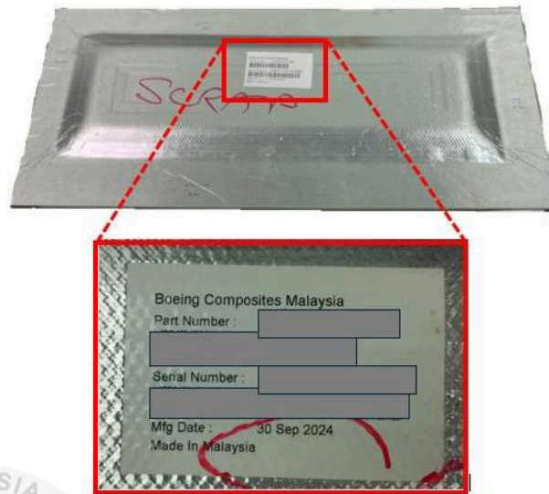
Figure 3.1: HFRP panel from Boeing Composites Malaysia
