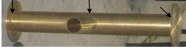
Figure 3.5: Showing that the area probability leakage for one sample of cylinder pipe.
