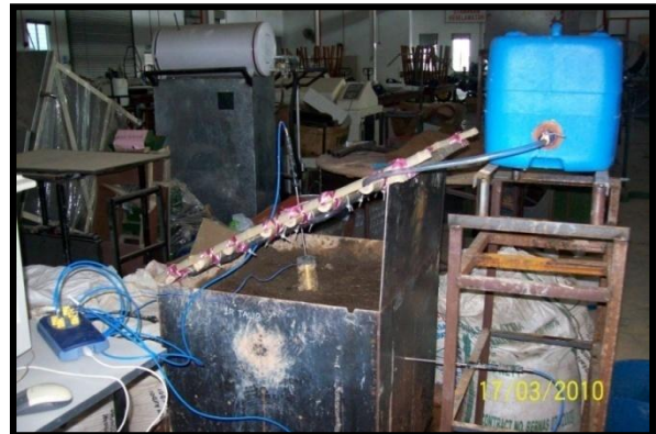
Figure 3.4: Water dripping system to simulate the water existance in the soil.
