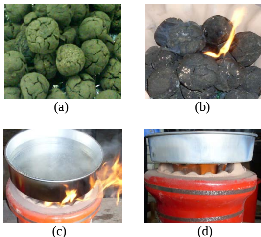
Fig 3: Photograph of (a) sample of DDC110, (b) initial combustion of DDC110, (c) flame of DDC110, and (d) flame of CHA.
