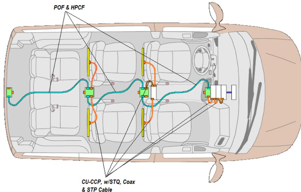
Figure 2 Physical Layer in 1394 Standard [15]
