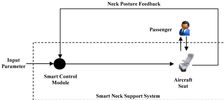
**Figure 4.** Feedback loop for smart neck support system.
