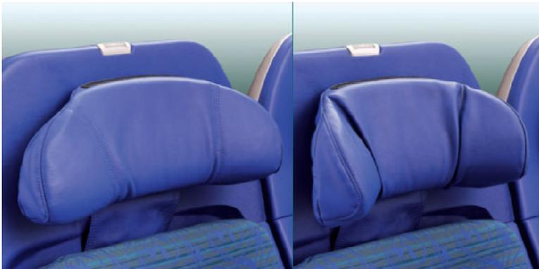
**Figure 3.** The Cathay Pacific Airlines economy class aircraft seat with built-in neck support (Photograph reprinted from [3]).
