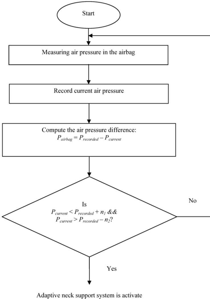
**Figure 13.** Flowchart for the neck support state transitions when the passenger is touching the airbag.
