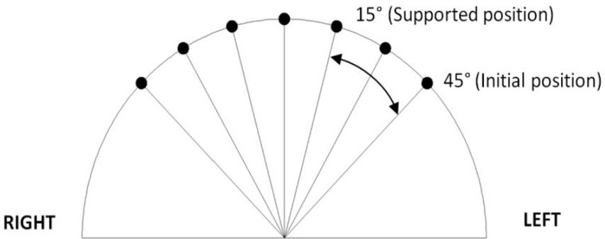
Figure 12. The schematic of example initial position and supported position for left airbag.
