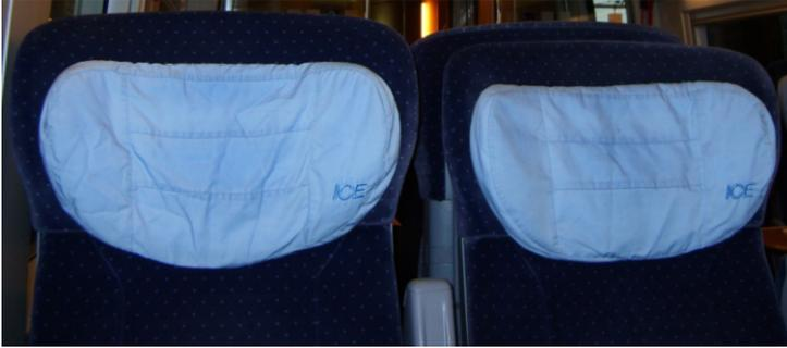
**Figure 2.** The German train ICE passenger seat with neck support.
