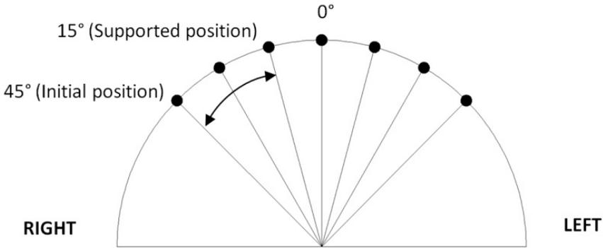
Figure 10. The schematic of example initial position and supported position for right airbag.
