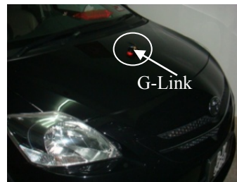
Figure 10 G-Link is mounted on the Toyota Vios car
