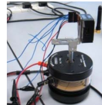
Figure 3 G-Link node and ADXL 321 mounted on the shaker stand
