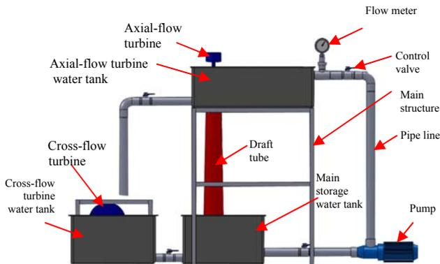
Fig. 1 Schematic diagram of test-rig
