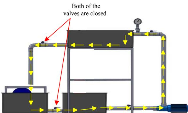
Fig. 3 Direction of water flows for experiment 2
