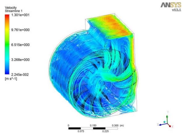
Fig. 8 CFD data analysis for mass flow rate of 40 l/s under cross-flow turbine
