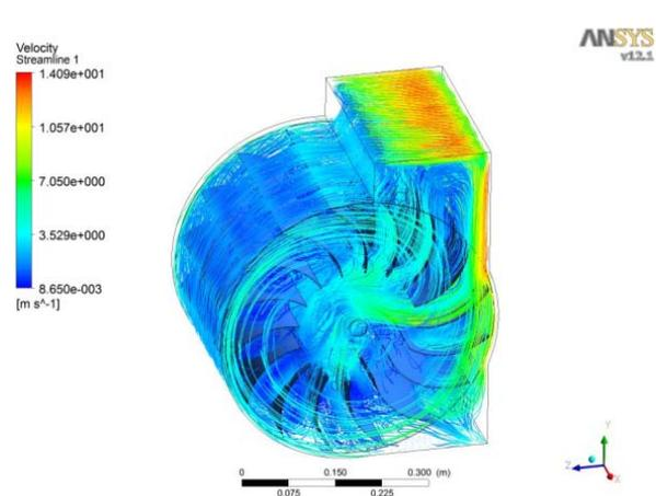
Fig. 9 CFD data analysis for mass flow rate of 50 l/s under cross-flow turbine
