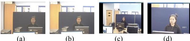
Figure 5. Image taken by the intelligence surveillance system. (a) Image taken by left IP camera; (b) Image taken by right camera; (c) The PTZ captured the targeted object; (d) The object zoom by ratio of 5.
