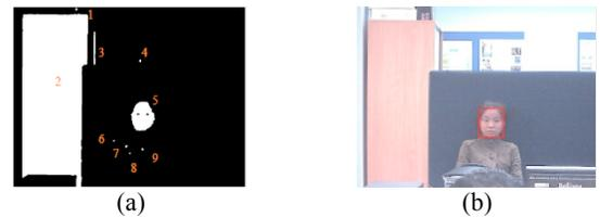
Figure 2. Morphological processing and connected region analysis. (a) Image after morphological processing. (b) Region of interest
