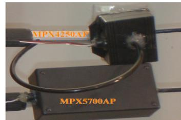
(b) System 2: Integrated Silicon Pressure Sensor
