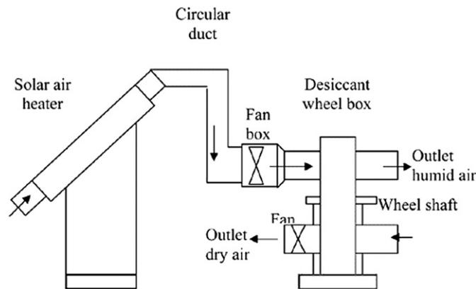
Fig. 20. Test loop for the desiccant wheel [34].
