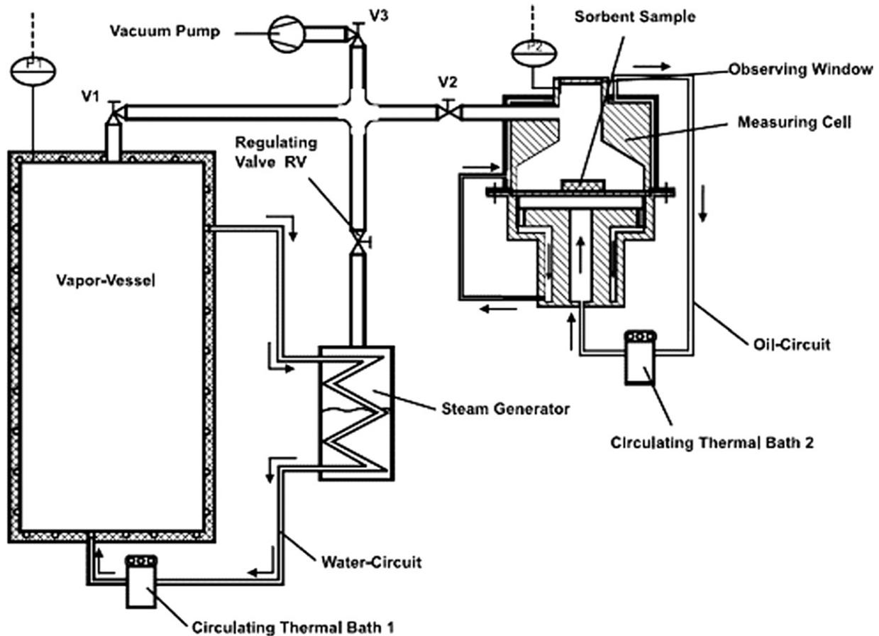
Fig. 38. Test-rig for measuring the kinetics of water vapor sorption [57].
