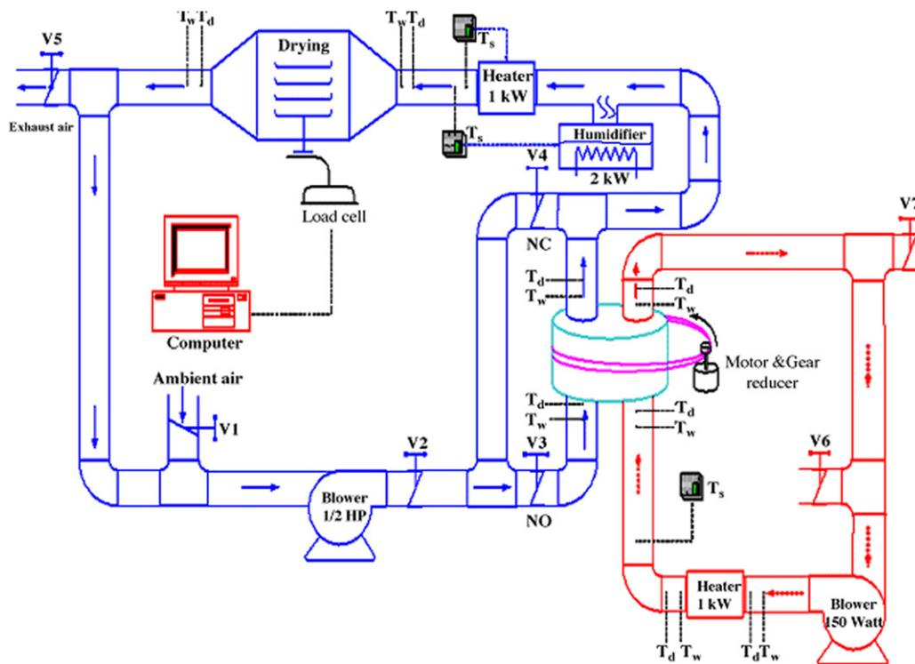
Fig. 10. Hot-air dryer integrated with rotary desiccant wheel [23].
