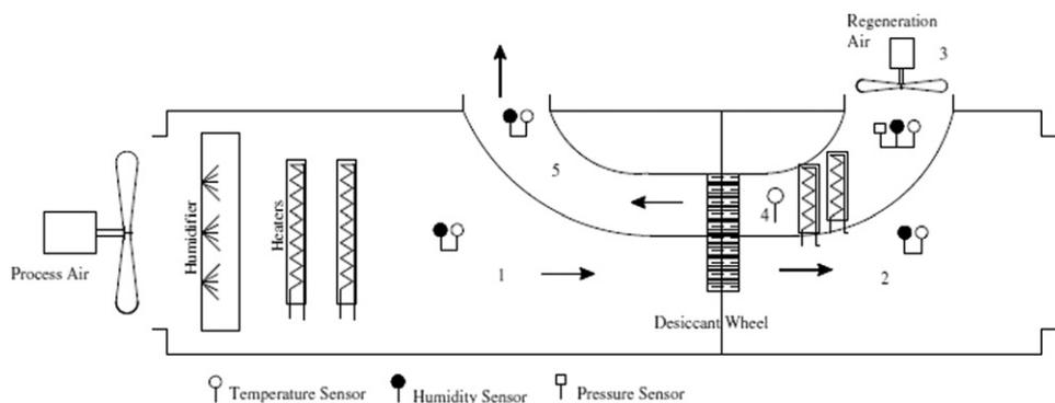
Fig. 23. Desiccant wheel experimental setup [37]. 1—Inlet process air; 2—outlet process air; 3—ambient air; 4—inlet regeneration air; 5—outlet regeneration air.
