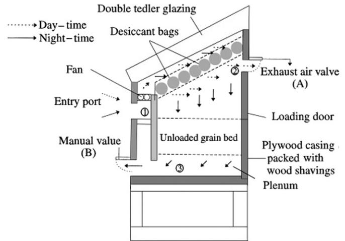
Fig. 9. Integrated desiccant/collector dehumidifier [22].
