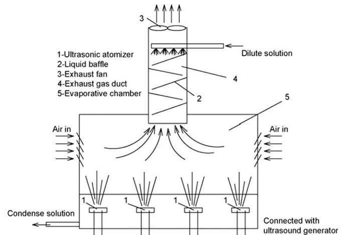
Fig. 27. Ultrasonic regenerator for liquid-desiccant [40].
