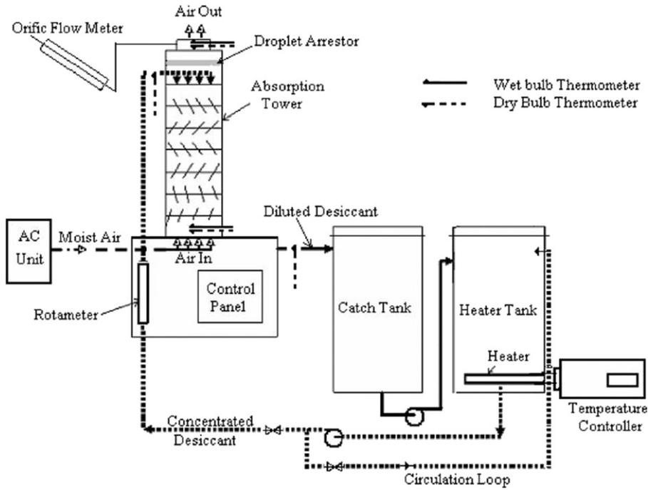
Fig. 33. Experimental setup for dehumidifier performance [50].
