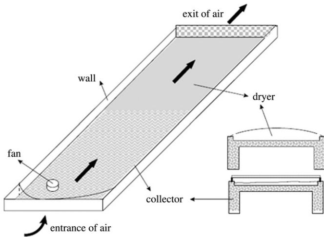
Fig. 6. Tunnel type dryer [20].
