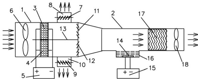
Fig. 26. Ultrasonic regenerator for solid desiccant [40].
