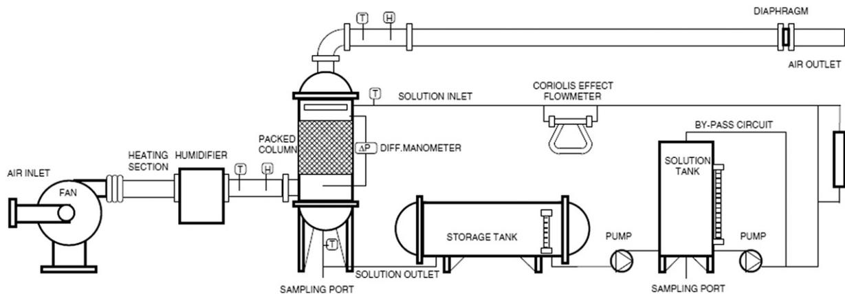
Fig. 39. Experimental setup of packed column dehumidifier/regenerator for liquid desiccant [58].
