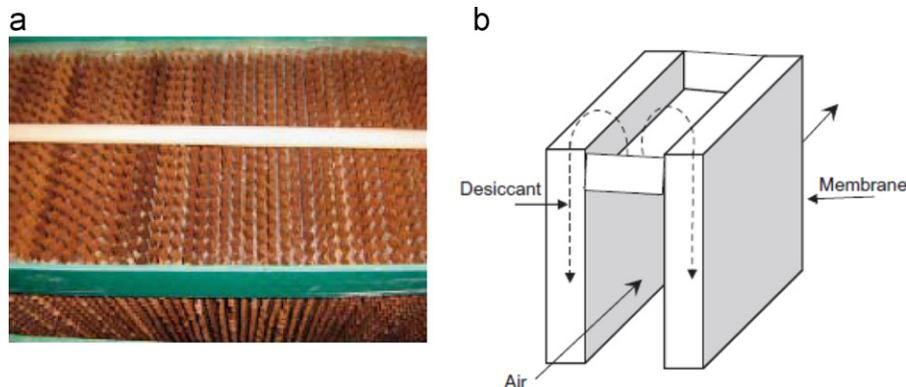
Fig. 41. Design of contactor [62]. (a) An inside view of the contactor in dehumidifier, (b) flow of desiccant and air inside the contactor.
