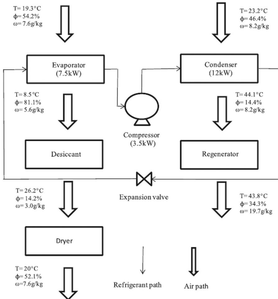
Fig. 17. Hybrid system drying air process [32].
