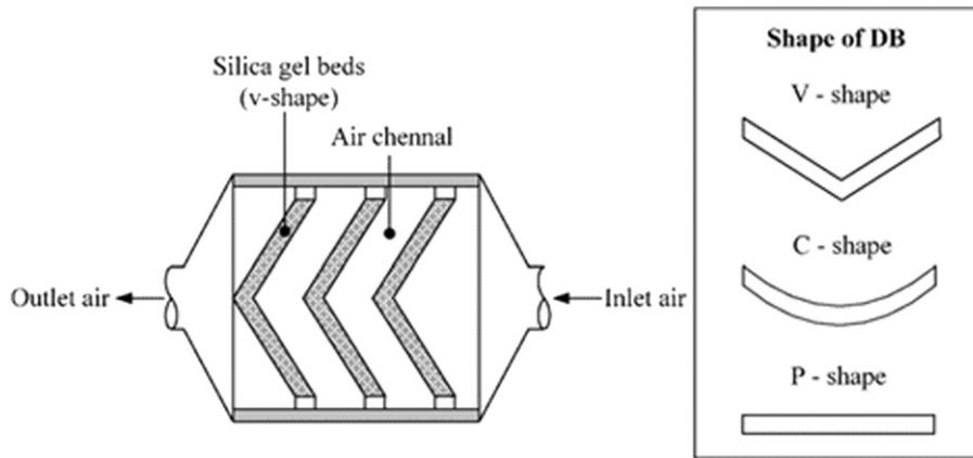
Fig. 13. Shapes of silica gel desiccant bed [24].
