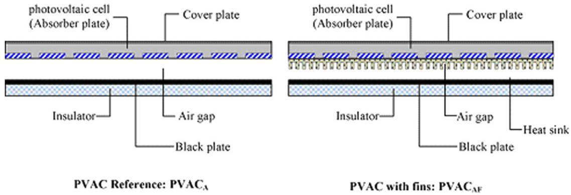
Fig. 12. Cross section view of PV/T air collector (PVAC) [24].
