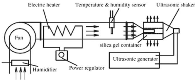
Fig. 25. Schematic diagram for power ultrasonic regenerator [39].
