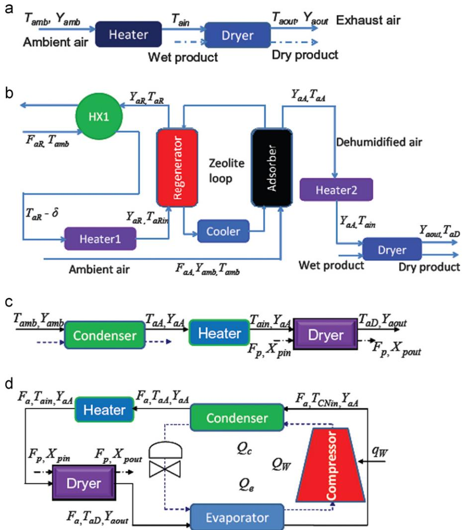
Fig. 1. Schematics of dryer types [12]. (a) Conventional dryer, (b) adsorption drying process, (c) condensation dryer and (d) heat pump dryer.
