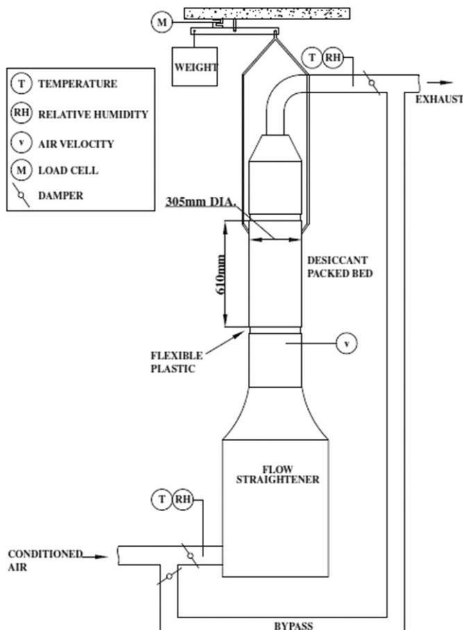
Fig. 35. Desiccant test setup [53].
