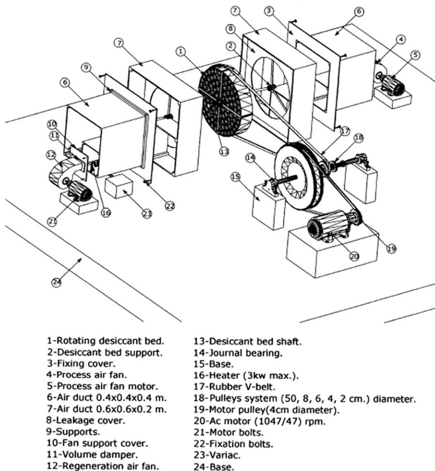
Fig. 32. Experimental setup of new rotating absorption disk [48].
