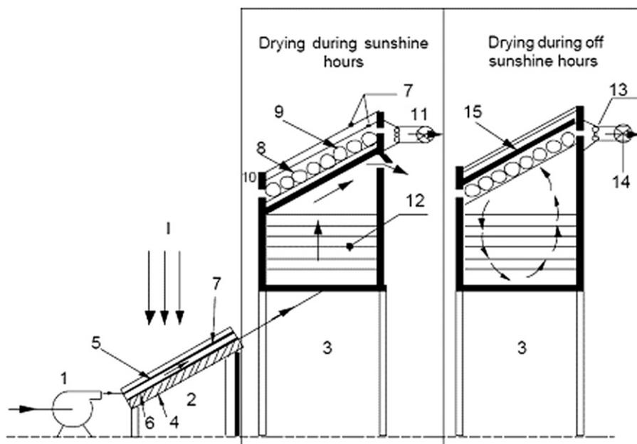
Fig. 5. Desiccant integrated solar dryer [18]. 1—Blower; 2—flat plate collector; 3—drying chamber; 4—insulator; 5—absorber plate; 6—bottom plate; 7—transparent cover; 8—desiccant bed; 9—plywood; 10—air inlet; 11—duct for air exit; 12—trays; 13—two-way fan; 14—valve; 15—plywood.
