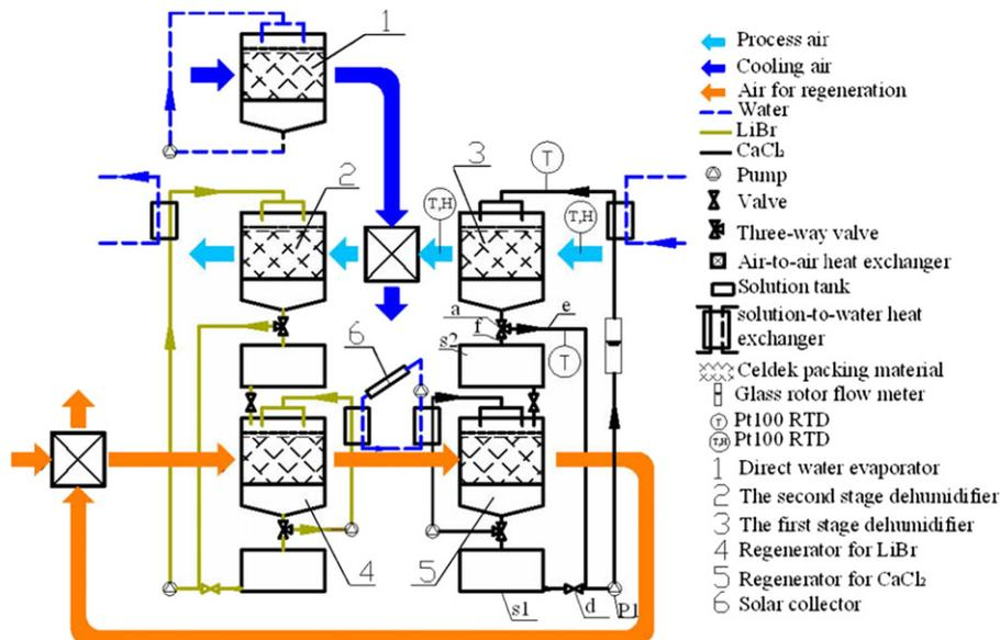
Fig. 21. Two stage liquid desiccant [35].
