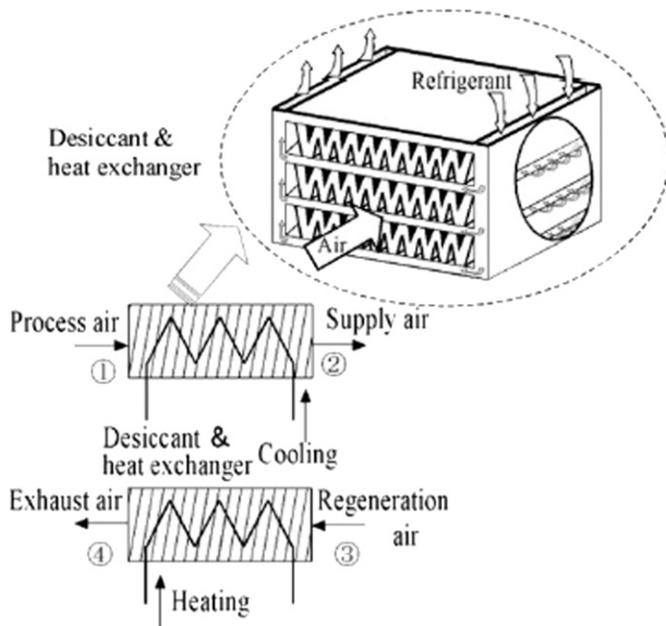
Fig. 3. Batch-type system with internal heat exchanger [15].
