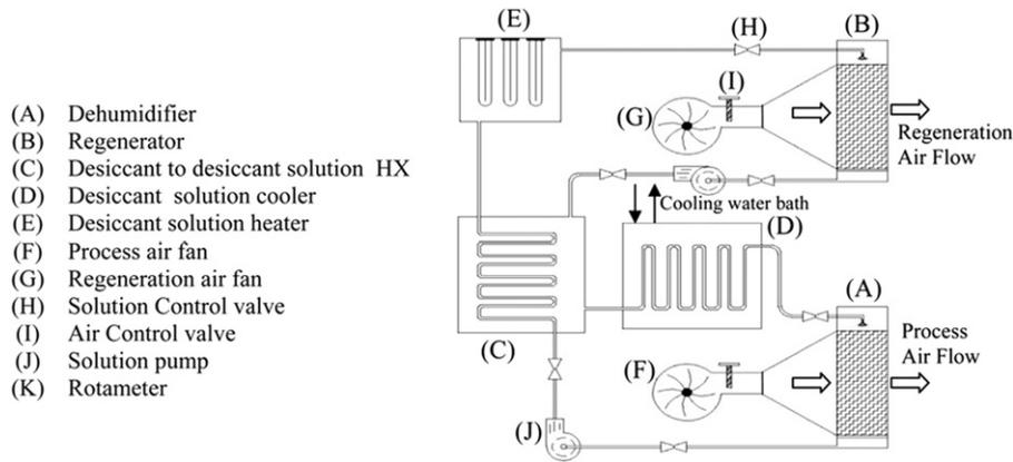
Fig. 24. Cross flow liquid desiccant dehumidification system [38].
