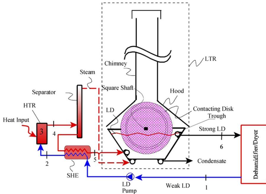
Fig. 14. LDBD with two-stage regenerator [27].
