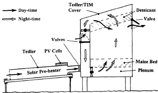
Fig. 4. Operation of solar-desiccant dryer [16].
