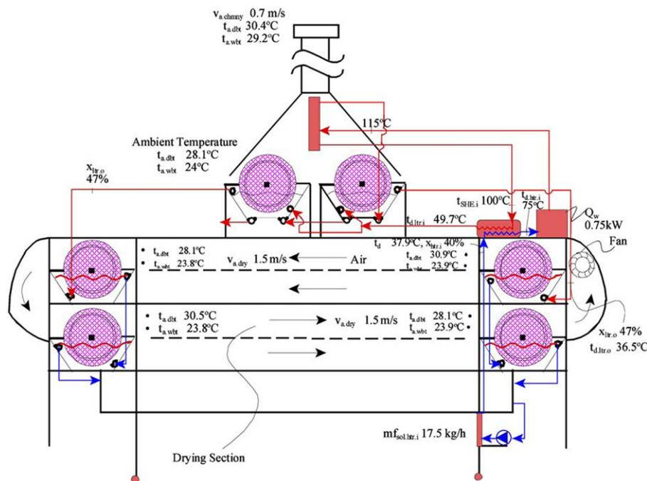
Fig. 15. Complete setup of LDBD [27].
