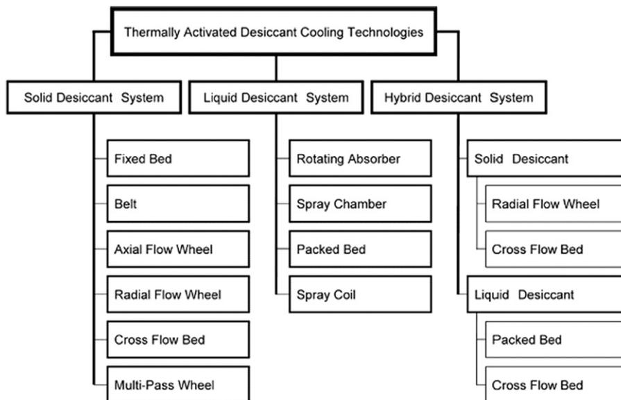
Fig. 2. Classifications desiccant cooling [13].
