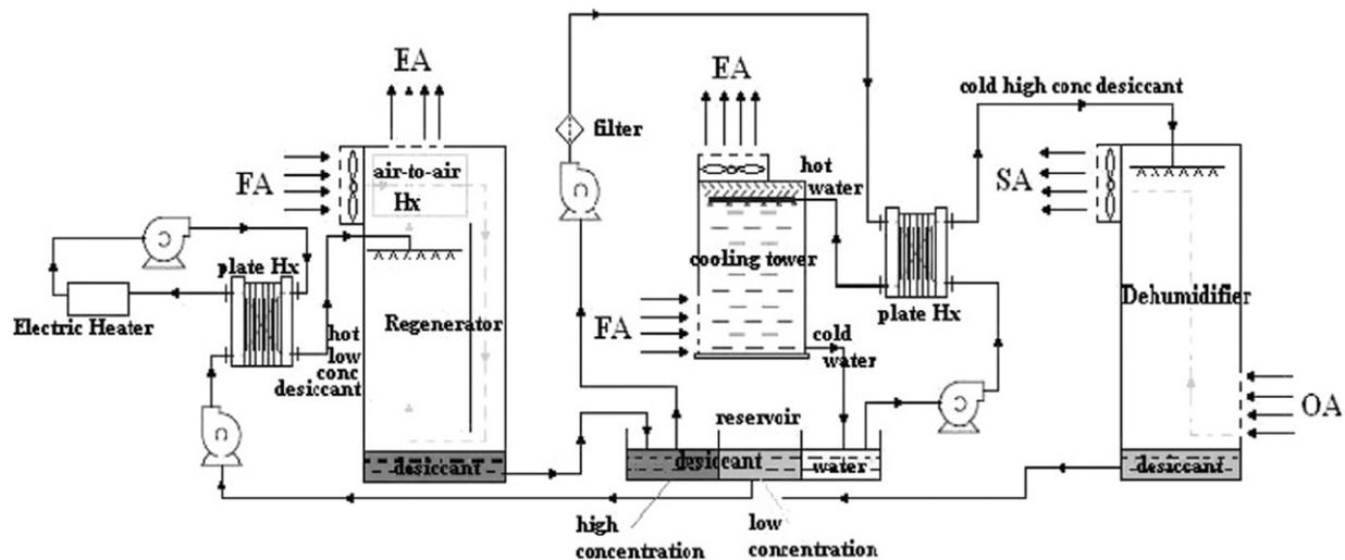
Fig. 40. Experimental setup for dehumidification system [62].
