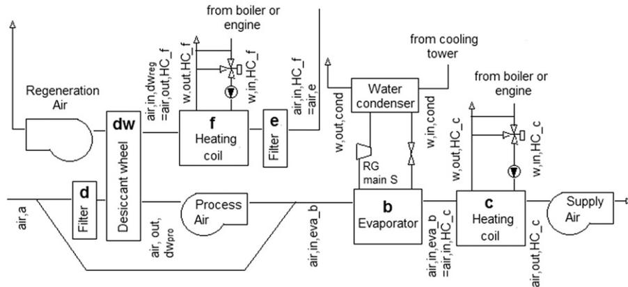
Fig. 29. Common desiccant wheel configuration [42].
