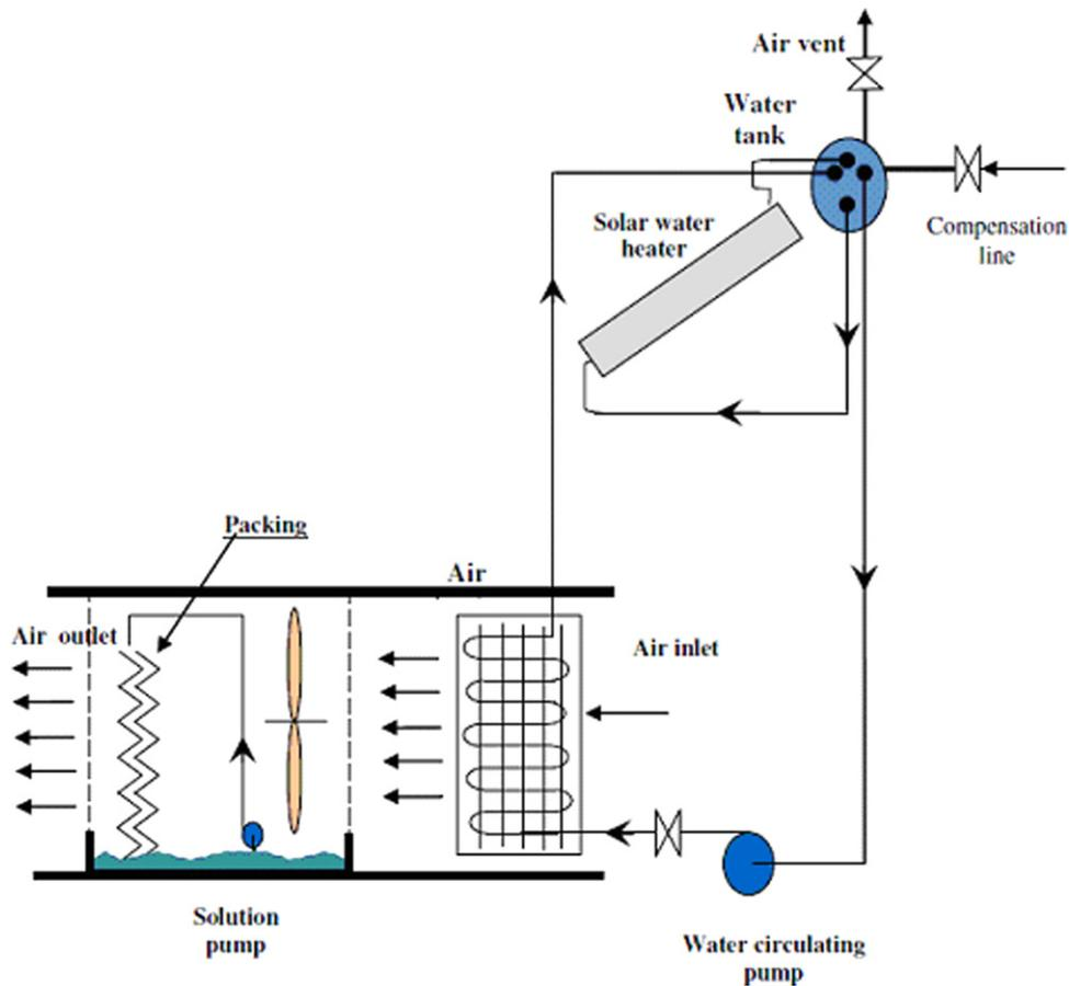
Fig. 22. Regeneration of liquid desiccant by solar energy [36].
