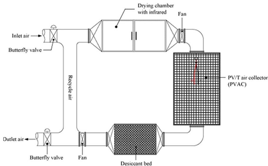
Fig. 11. Hybrid PV/T-desiccant integrated with infrared drying system (HPIRD) [24].
