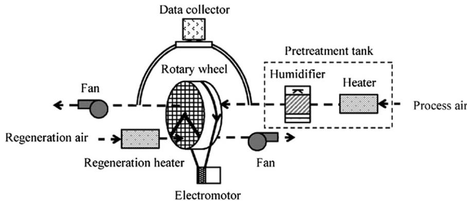
Fig. 37. Experimental set-up of adsorption test [55].
