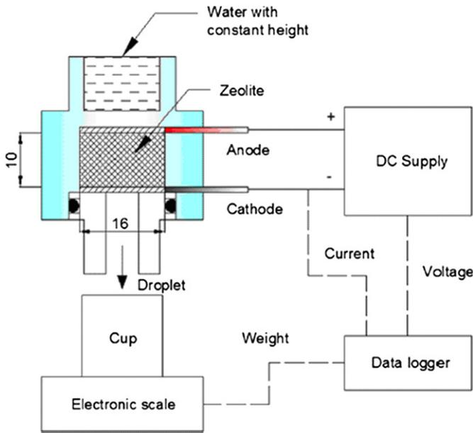
Fig. 30. Experimental setup of the EO regeneration system [44].
