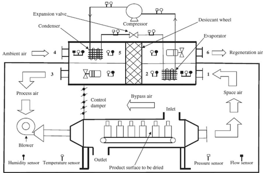
Fig. 16. Hybrid desiccant system [32].
