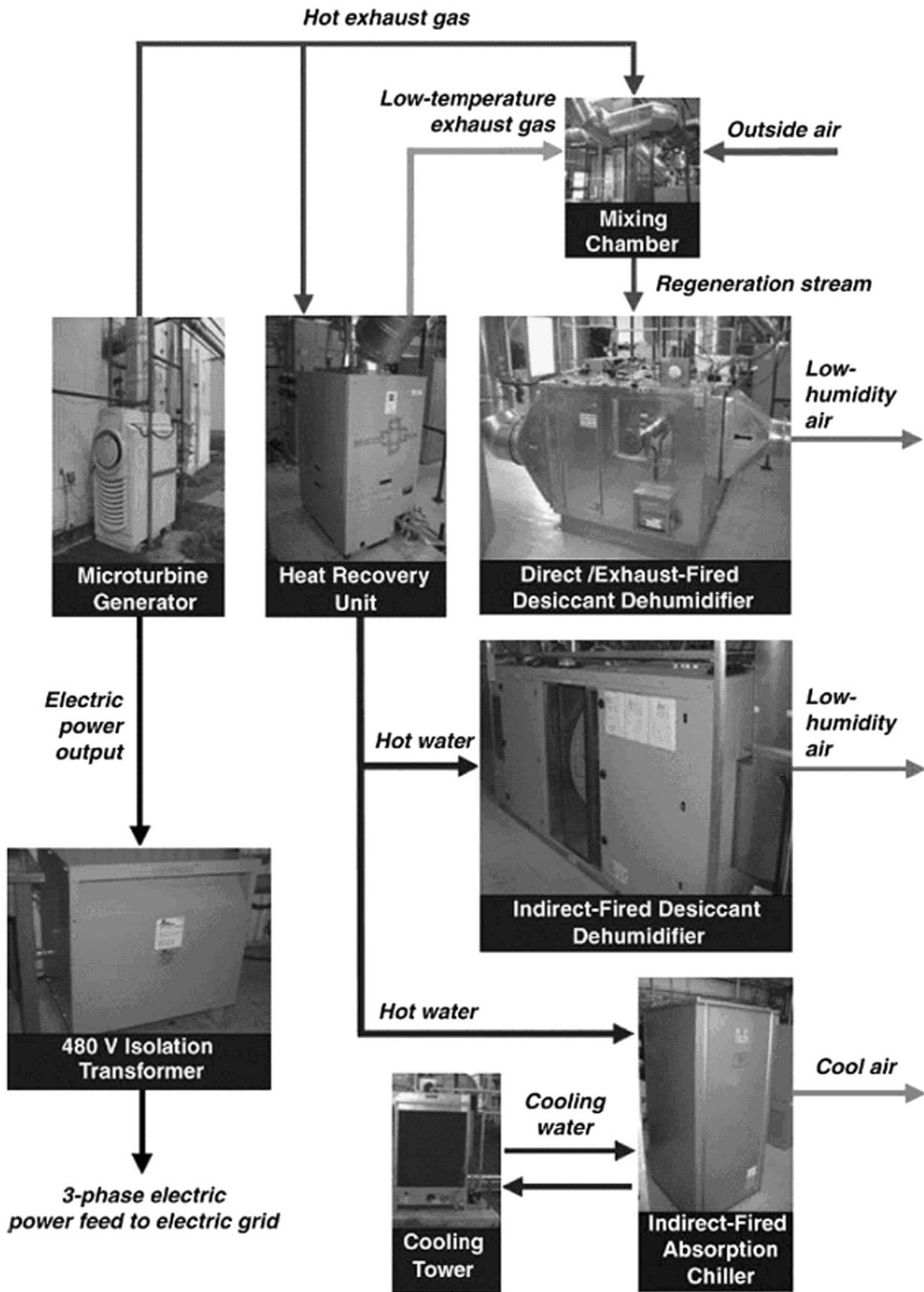
Fig. 28. Integrated Energy System [41].
