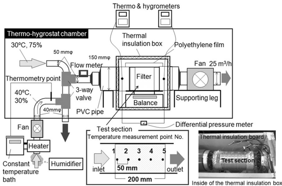
Fig. 36. Adsorption/regeneration test of WSS [54].
