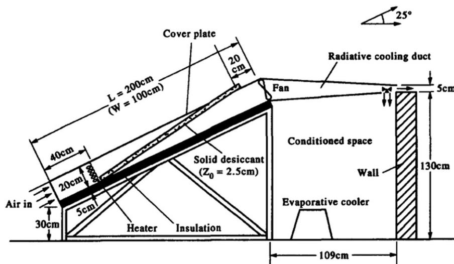
Fig. 18. Installation of SDERC system [33].
