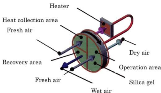
Fig. 8. Desiccant drying rotor [21].
