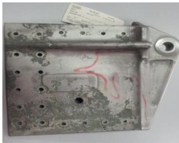
Figure 1: Pitting corrosion of Fitting sponson spar AFT, Nuri Helicopter
