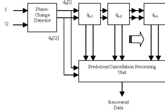
**Figure 4: Block diagram of multiple differential detection scheme**
