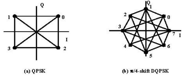
**Figure 1: The signal space of (a) QPSK versus the signal space of (b)  $\pi/4$ -shift DQPSK**
