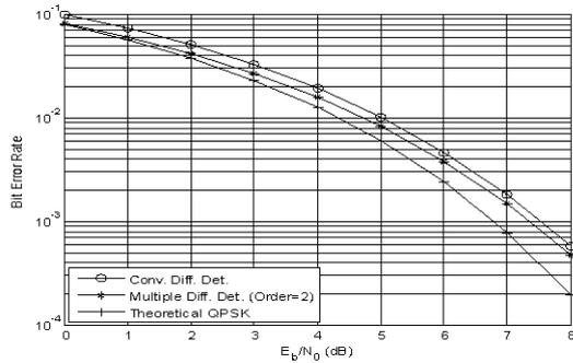
Figure 9: Performance comparison of conventional and multiple differential detection schemes in AWGN channel
