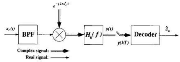
**Figure 3: Block diagram of receiver model**
