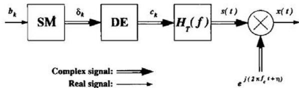
**Figure 2: Block diagram of transmitter model**
