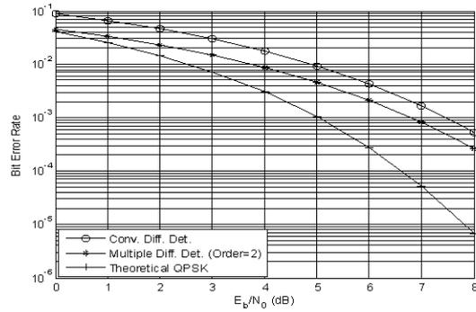
Figure 10: Performance comparison of conventional and multiple differential detection schemes in AWGN and Rayleigh fading channel
