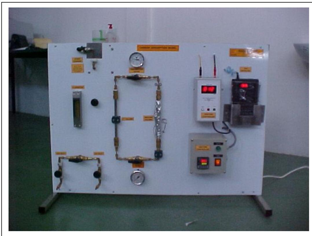
Fig. 2. Carbon adsorbent test bed
