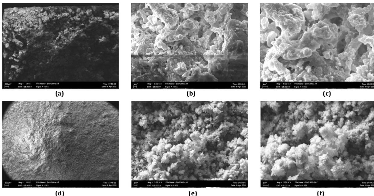
**Figure 3:** SEM images of ZnO at different temperatures and magnifications, (a) ZnO at 250°C, 20X, (b) ZnO at 250°C, 3000X, (c) ZnO at 250°C, 5000X, (d) ZnO at 500°C, 20X, (e) ZnO at 500°C, 3000X, (f) ZnO at 500°C, 5000X.
