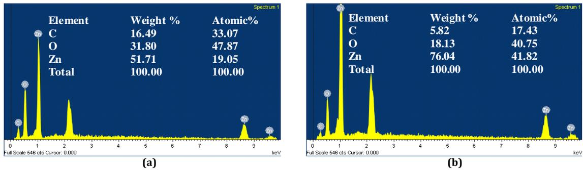
Figure 5: EDS spectra of ZnO at different temperatures, (a) 250°C, (b) 500°C.
