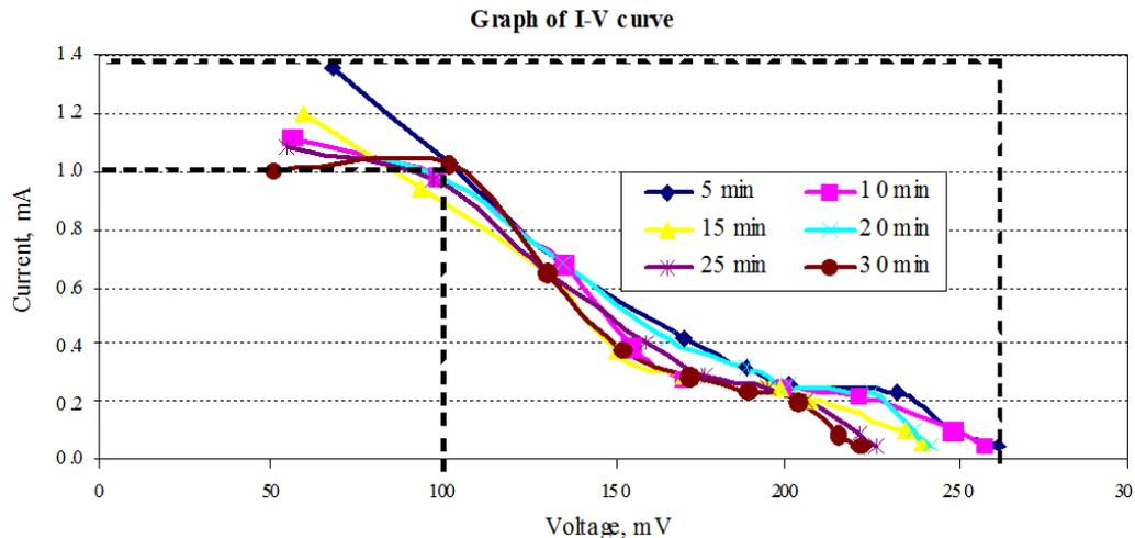
**Figure 7:** I-V curves for the fabricated DSSC using two ITO glasses with one electrode coated with graphite and the other coated with ZnO powder annealed at 500°C and treated with natural dragon fruit dye
