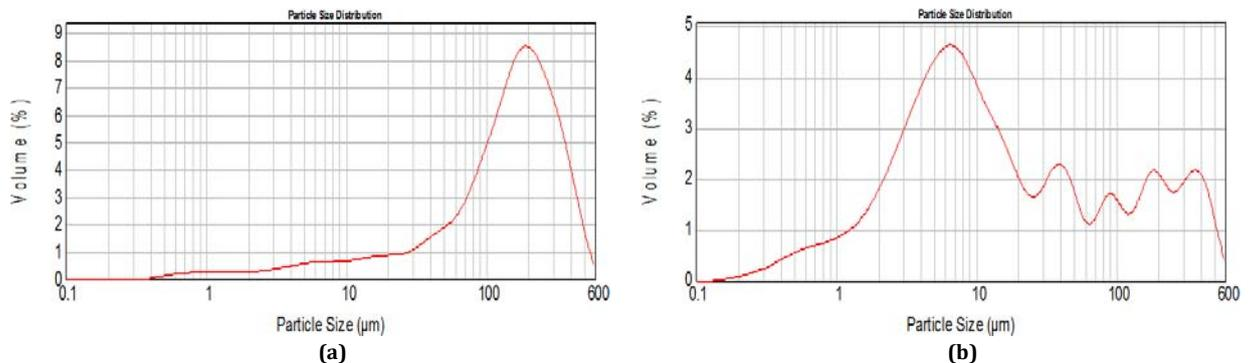
**Figure 2:** Particle size distribution of ZnO at different temperatures, (a)  $250^\circ\text{C}$ , (b)  $500^\circ\text{C}$ .
