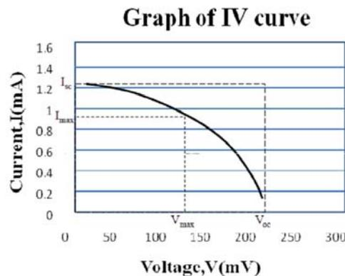
Figure 6: Theoretical graph of I-V curve showing  $I_{sc}$ ,  $V_{oc}$ ,  $I_{max}$  &  $V_{max}$  for determining  $P_{max}$  and  $FF$
