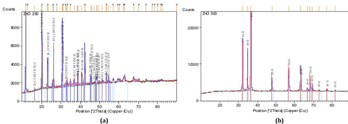
**Figure 4:** XRD patterns of ZnO powder at different temperatures, (a) 250°C, (b) 500°C.
