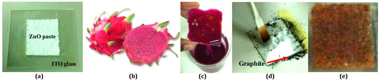
**Figure 1:** Preparation of the Dye Sensitized Solar Cell, (a) ZnO electrode preparation, (b) Fresh dragon fruit, (c) ZnO electrode coated with dragon fruit dye, (d) Counter electrode preparation, (e) Prepared DSSC.
